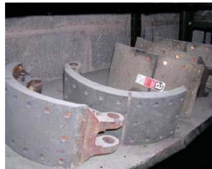
Figure 41 Asbestos brake linings for quarry vehicles
