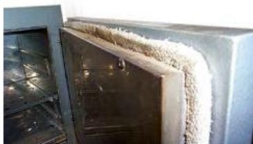
Figure 26 Asbestos rope seal on drying oven
