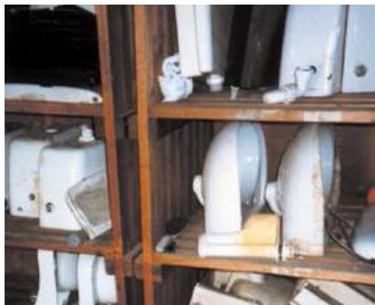
Figure 40 Asbestos-reinforced toilet cistern
